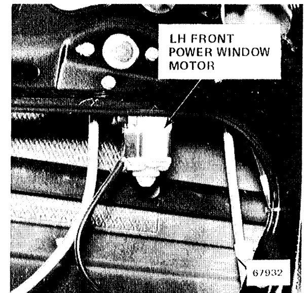
Figure 6 - Inside LH Front Door (Panel Removed)
